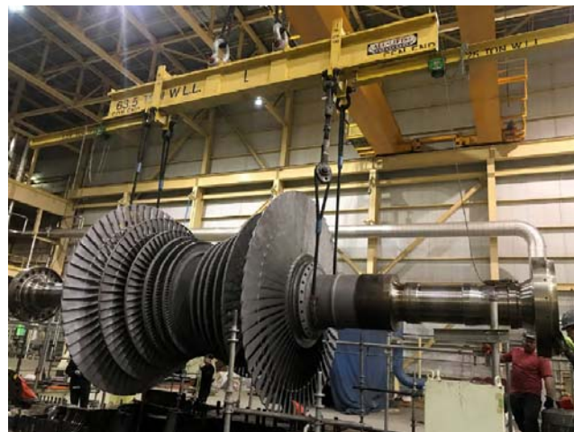
Figure 3. Comanche 3 low pressure B (LPB) rotor.
