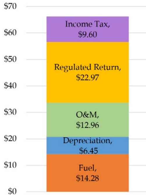
Figure 28. Comanche 3 LCOE components ($/MWh), 2010-2020.
